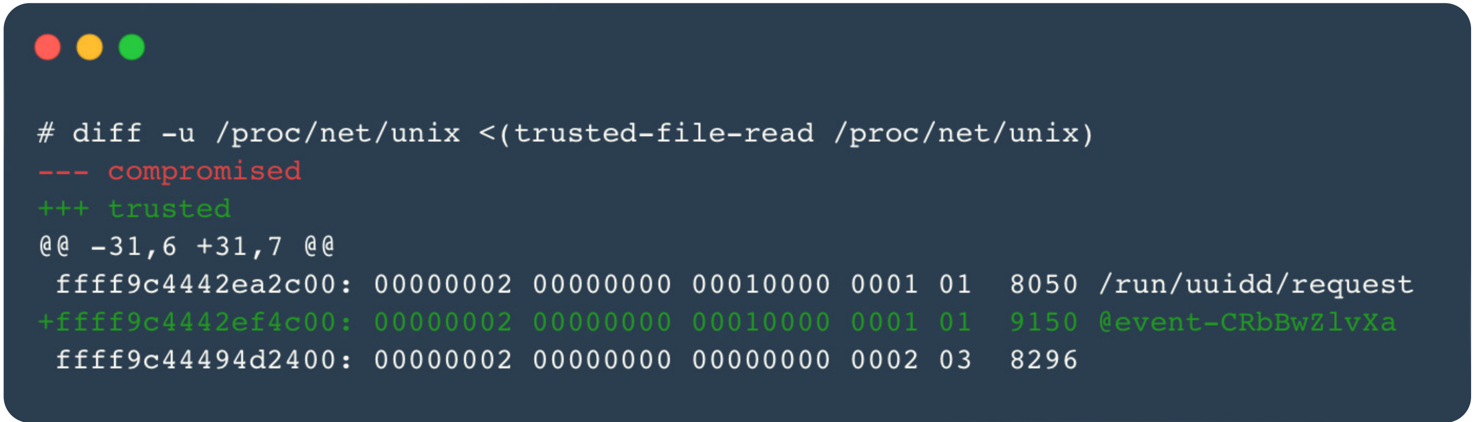
Figure 17. Difference between /proc/net/unix seen under a program compromised with Ebury and one that is not
