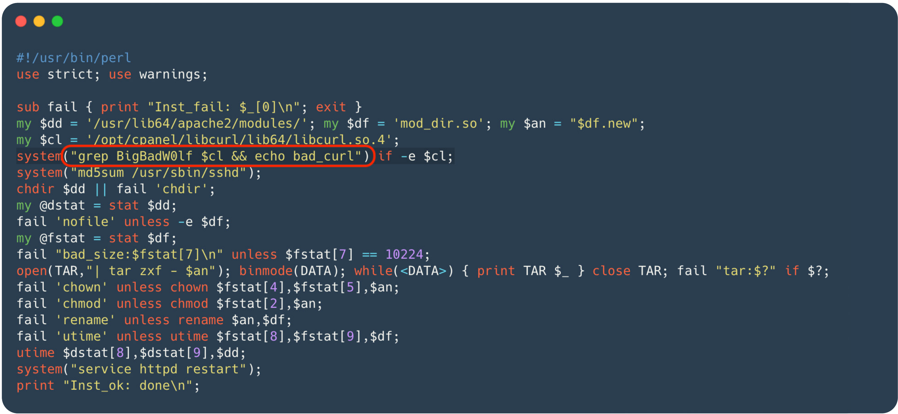
Figure 6. HelimodSteal installation script with detection of the string BigBadW0lf in libcurl.so.4 highlighted
